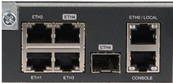
Figure 2-16. View of the network management communication interfaces.
