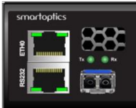
Figure 12. Network management communication interfaces in the front of the DCP-M32-CSO-ZR+ and DCP-M40-MSO-ZR chassis.
