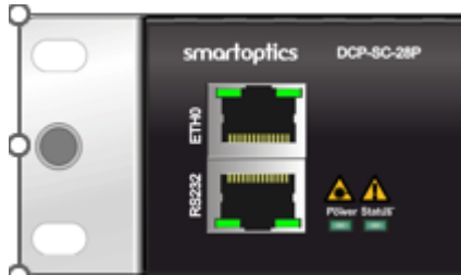
Figure 7. Network management communication interfaces in the front of the DCP-SC-28Pchassis.
