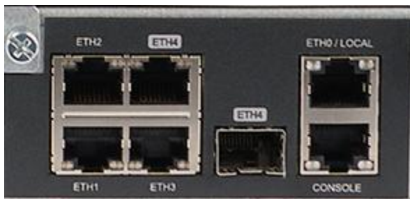
Figure 10. Network management communication interfaces in the back of the DCP-M40 chassis.
