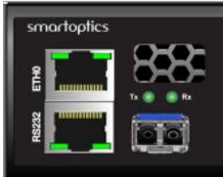
Figure 12. Network management communication interfaces in the front of the DCP-M32-CSO-ZR+ chassis.
