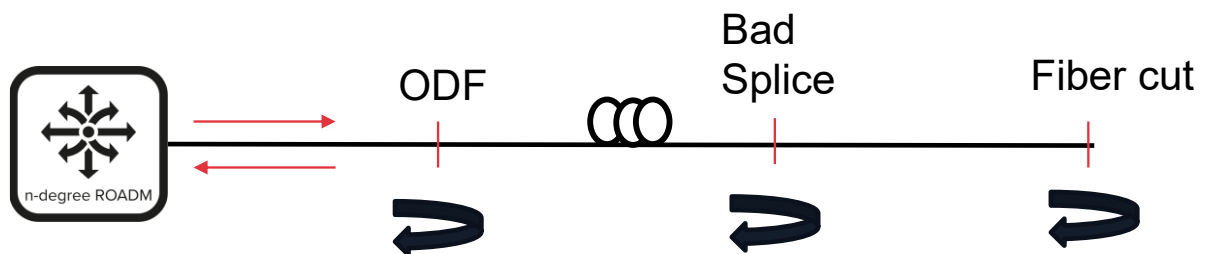
Figure 39. Example of reflection points in OTDR measurements
